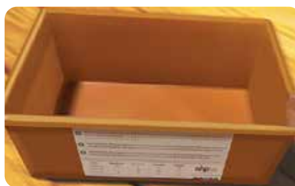
OHP calibration pan with directions for use sticker
